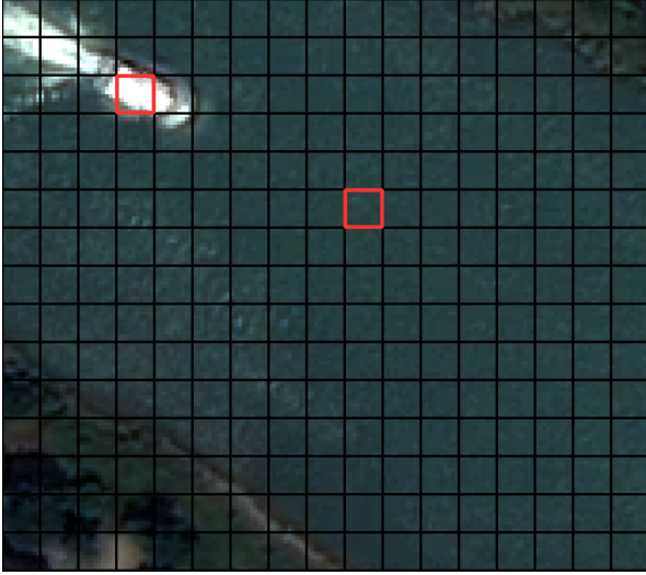
Figure 5: Detailed view of the chessboard segmentation, in black, and selection of two segments, in red.
